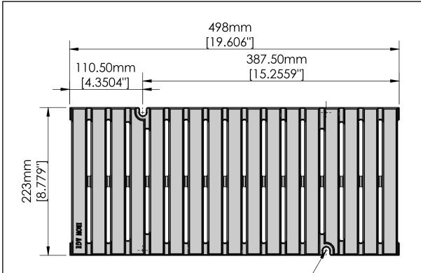
(2x) slot for M8 button head screw, locations correspond w/bolt-dn holes in MEADRAIN™ channel
