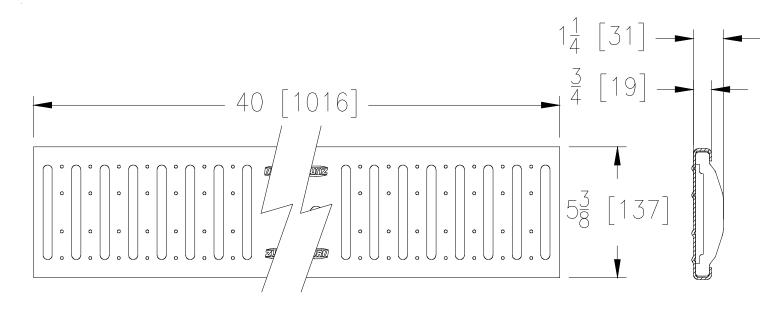
**RFG GRATE ENGINEERING SPECIFICATION:** The Zurn P6-RFG, Reinforced Slotted, Galvanized Steel Grate, is 5.375 inches wide by 40 inches long, weighing 4 lbs per linear foot. The grate has an open area of 12 square inches per linear foot, DIN Rating of B, ANSI Rating of Medium Duty. Galvanizing conforms to ASTM specification A653, Galvanized Coating designation G60, minimum spangle.
