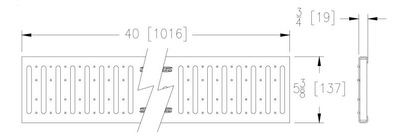
**FS GRATE ENGINEERING SPECIFICATION:** The Zurn P6-FG, Slotted, Stainless Steel Grate, is 5.375 inches wide by 40 inches long, weighing 1.7 lbs per linear foot. The grate has an open area of 12.0 square inches per linear foot, DIN Rating of A, ANSI Rating of Light Duty.
