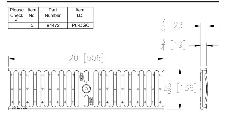
**DGC GRATE ENGINEERING SPECIFICATION:** The Zurn P6-DGC, Slotted Grate, Ductile Iron Grate, is 5.375 inches wide by 20 inches long, weighing 4.5 lbs per linear foot. The grate has an open area of 28.1 square inches per linear foot, DIN Rating of C, ANSI Rating of Heavy Duty, H-20 Load Rated.
